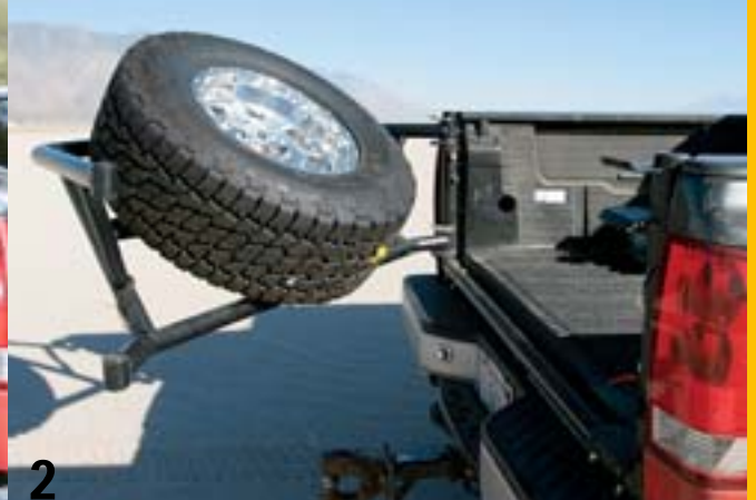
2 The TireGate is the perfect balance between functionality and good looks. The sweetest part about it is that it doesn't require any cutting, drilling, or welding to mount. It required just 10 bolts, making this product truly bolt-on. We also installed a cable-style bike lock to prevent spare-
