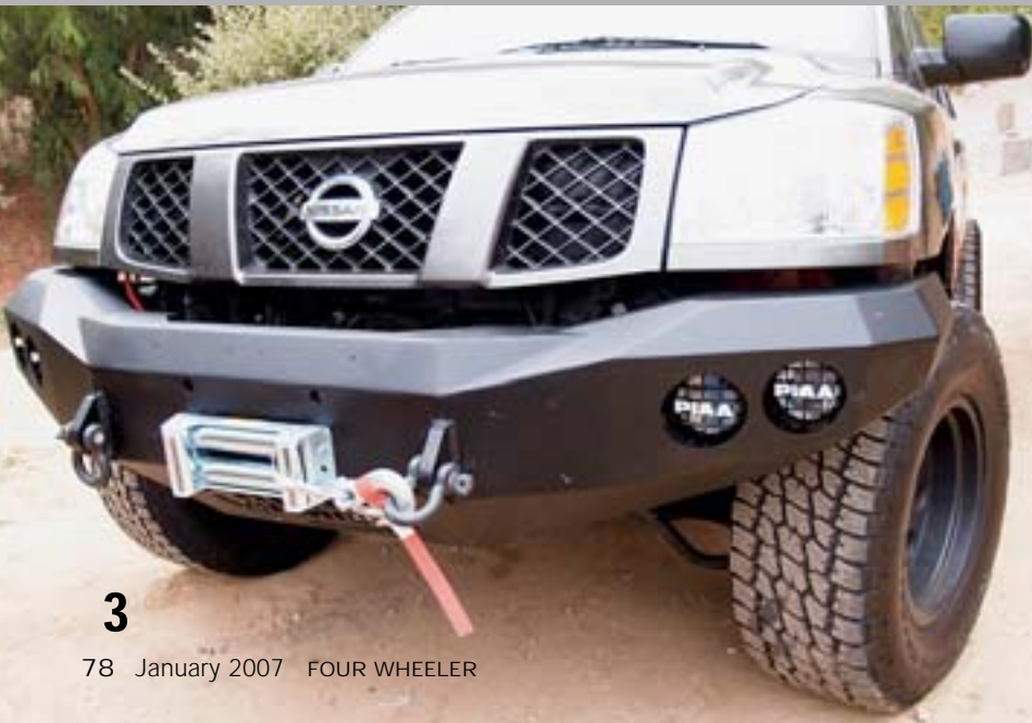
3 This is the newest bumper in road Armor's lineup. It came to us strapped to a large wooden pallet, powdercoated black, with some of the necessary hardware to install it. Unfortunately, we did have to make a run to the local hardware store for four fine-thread metric bolts to complete the installation. Notice the gap between the lower portion of the grille and the top of the bumper. We didn't exactly like this aspect of the bumper, but felt we could live with it
