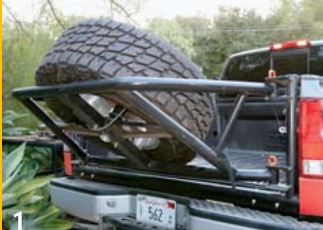
1 Here is the TireGate in the closed position. We decided to run it with the tire positioned outward so as to improve bed-cargo capacity. Every TireGate is powdercoated with black polyester semi-gloss and is equipped with zinc-plated hardware for long-lasting good looks.
